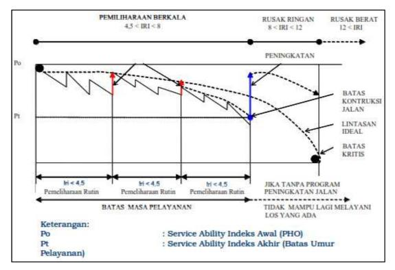
Figure 2: Relationship Between Condition, Age and Types of Road Handling [21]
